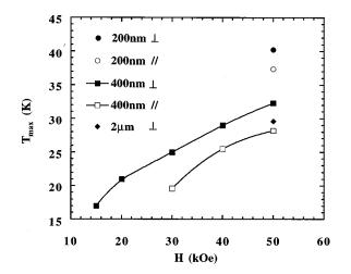
FIG. 3. The dependence of resistance maximum  $T_{\text{max}}$  on magnetic field for various wire diameters, where solid and open symbols stand for transverse ( $\perp$ ) and longitudinal (||) field geometry, respectively.
