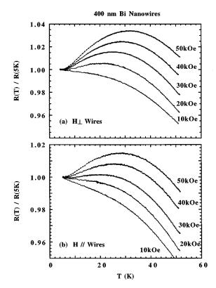
FIG. 1. Temperature dependence of (a) resistance and (b) magnetoresistance of the 400-nm Bi nanowires, with and without a magnetic field of 50 kOe applied perpendicular and parallel to the wires.
