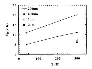
FIG. 5. Temperature dependence of the deviation field  $H_D$  for various wire diameters.
