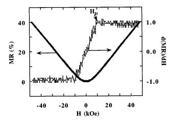
FIG. 4. Representative magnetic field dependence of (a) magnetoresistance and (b) d(MR)/dH for 400-nm Bi nanowires, with the deviation field  $H_D$  indicated.
