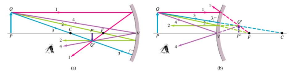
Ray 1 goes out from Q parallel to the axis & reflects through F.
