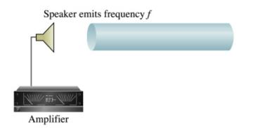
When the driving frequency equals a normal mode frequency of the system, energy will be added into the system and increase the oscillation amplitude.
