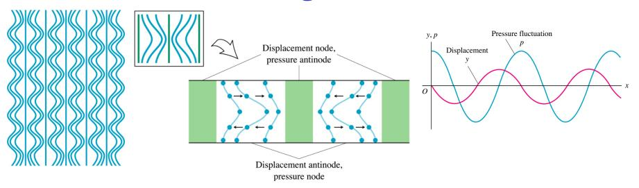
Displacement node: where particles have zero displacement
