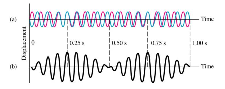
Beats: Periodic amplitude variations caused by two waves with slightly different frequencies.
