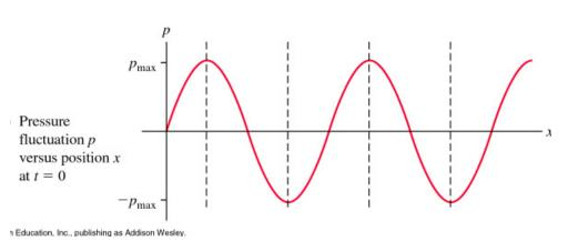
Pressure fluctuation extremes Zero displacement Zero pressure fluctuation Displacement extremes Liu UCD Phy9B 07
